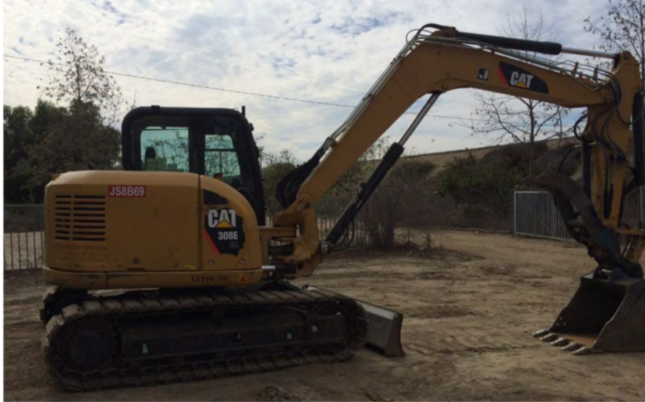
PHOTO 3: EXCAVATOR WITH BUCKET & GRAPPLE
